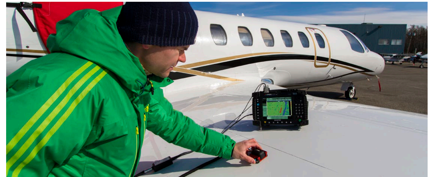
For maximum detection, the MXB software features 8-frequency scanning and amplitude and phase C-scan display.
