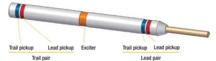
The dual pickup acts as two single-exciter probes in one probe casing, combining the excellent wall-loss response of the ABS channel with the dual-exciter model's capability to detect pits on each side of the support plate. This makes the dual-pickup model ideal for inspecting both tube sheets.
