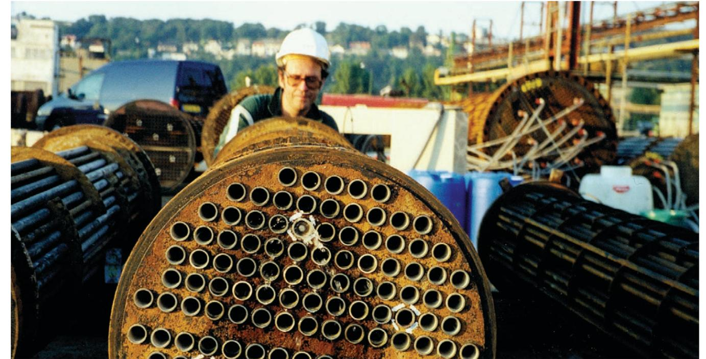
The internal rotary inspection system (IRIS) is an ultrasonic technique well suited to petrochemical and balance-of-plant (BOP) tube inspections. This technique uses an ultrasonic beam to scan the internal surface of the tube in helicoidal patterns, thus ensuring that the full length of the tube is tested. Olympus tube inspection systems monitor the front-wall and back-wall echoes to measure the tube wall thickness.
