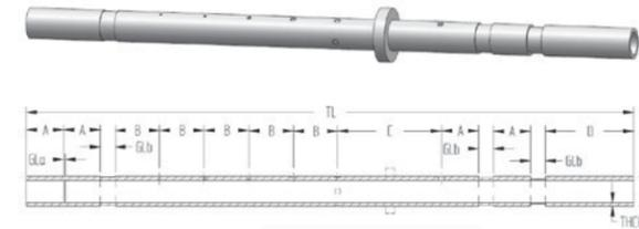
CT02 — ECT Extended ASME calibration tube.
