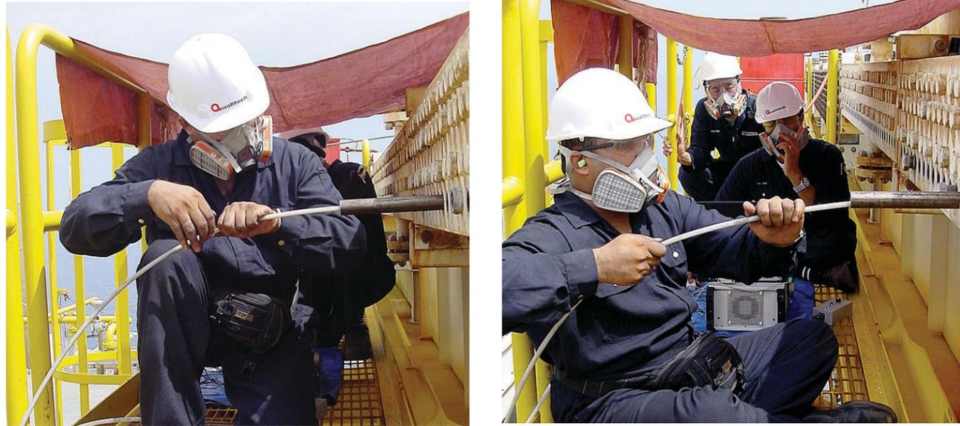
The magnetic flux leakage (MFL) technique is based on magnetization of the material being inspected. Magnetization is provided by a strong magnet located inside the probe. As the probe encounters a wall reduction or sharp discontinuity, the flux distribution varies around that area and is detected either with a Hall-effect transducer or an inductive pickup coil.
