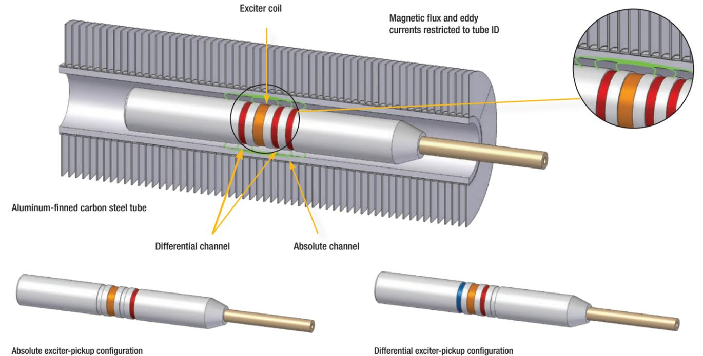
The absolute channel easily detects internal volumetric defects, such as corrosion, erosion, and wall thinning. The damage severity can be evaluated by exclusively analyzing the signal amplitude.
