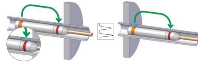
Large defect detected from the ABS channel on both sides of the support.
