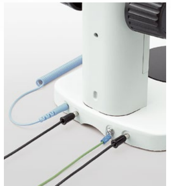
Ground wire connection (back side)
