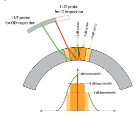
When two conventional UT probes are used on each side of the weld (one for ID and one for OD inspection), only a very narrow zone in the center of the HAZ is covered at 0 dB attenuation due to the UT probe's beam width profile. Slight mechanical movement (positioning) can result in high variations of the detection amplitude.
