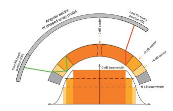
Using only one PA probe on each side of the weld provides wide sector coverage of the heat-affected zone (HAZ) with constant amplitude. This unique solution provides constant amplitude detection within the entire inspection area, even when there is significant mechanical movement (positioning).
