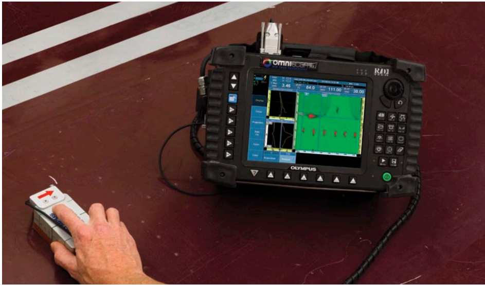
Display showing C-scan, impedance plane, and strip chart views. Note that the doubler edge and rivets are clearly visible.
