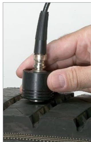
Measure depth to steel ply / cords in rubber conveyor belts or tires.
