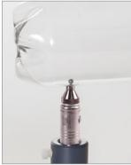
In applications such as plastic containers, simply drop the small target ball inside the container. The magnetic probe held on the outside of the container attracts the target ball. When scanning the probe along the surface or critical corners, the small steel target ball will follow. In the Minimum Mode feature, the gauge continually
