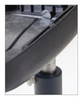
The standard probe along with one of the two target disks and a replaceable chisel wear cap makes the Magna-Mike 8600 gauge ideally suited for most automotive tear seam applications where measurements need to be made in a thin channel or groove.
