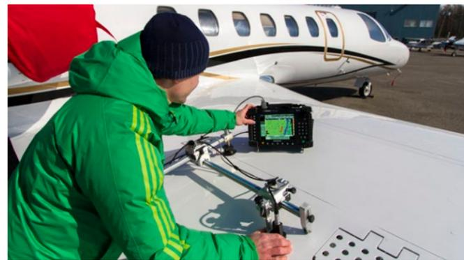
Encoded system: any two-axis encoding scanner can be used to inspect a part. Olympus offers two options: the GLIDER™ scanner, which is well-suited for flat or slightly curved surfaces, and the WING™ scanner, which is specially designed for scanning curved parts (e.g., aircraft fuselages) and can even be used upside-down due to its Venturi vacuum-cup system. For more versatility, a handheld one-axis encoding scanner, equipped with an Indexer Clicker, is also compatible with this system.
