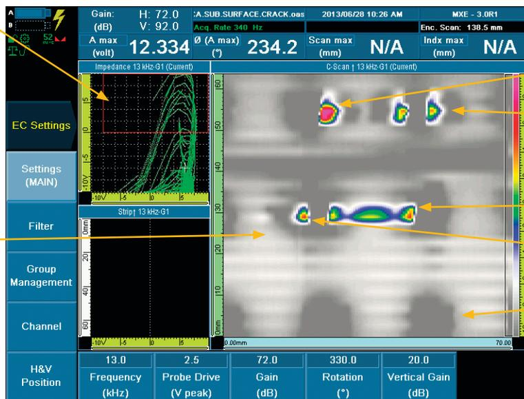
Detailed subsurface crack ECA imagery
