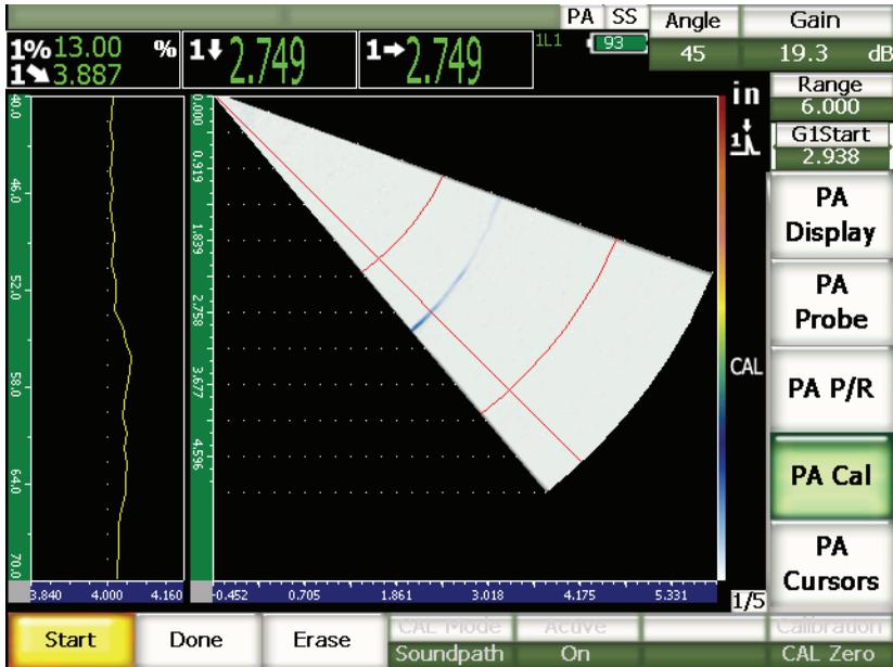
Figure 17-20 The Wedge Delay acquisition screen
