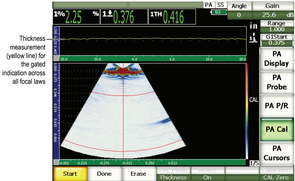
**Figure 17-7 The Wedge Delay acquisition screen with thickness measurement reading at the top**
