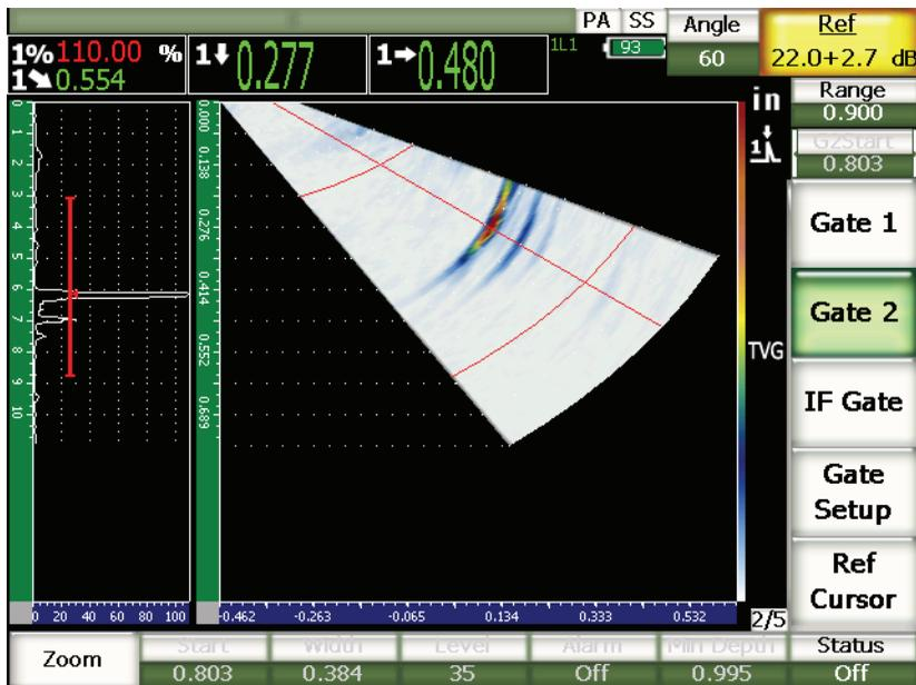
Figure 15-1 A-scan and S-scan with viewable gate
