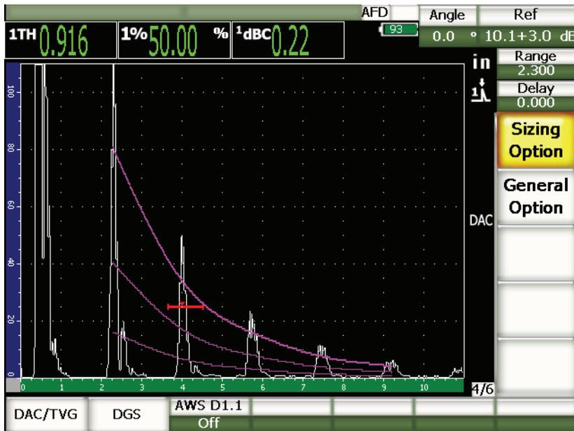
Figure 11-11 ASME DAC with 3 dB scanning gain and reference correction active
