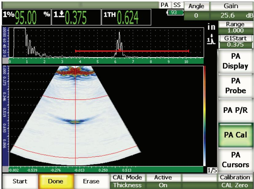
Figure 17-8 A completed wedge delay calibration
