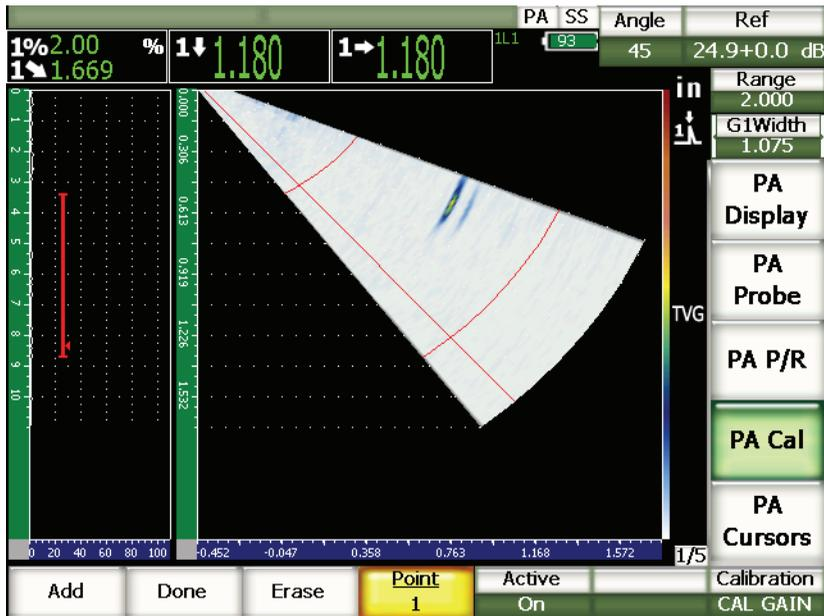
Figure 17-24 The completed gain calibration
