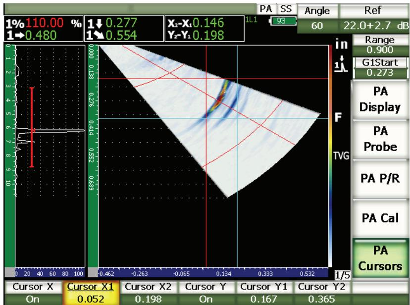
Figure 16-2 Cursors on S-scan with measurement
