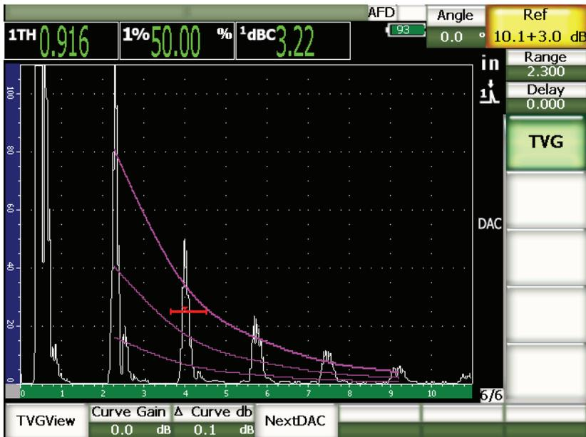
Figure 11-10 ASME DAC with 3 dB scanning gain
