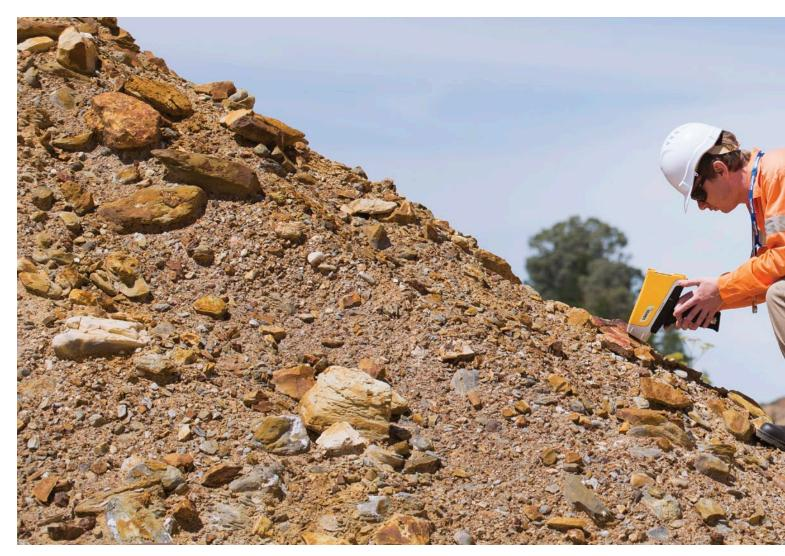
The Olympus Vanta<sup>™</sup> handheld XRF provides immediate, on-site elemental measurements for a range of geochemical applications. Vanta analyzers provide power and flexibility across the entire mineral resource cycle:
