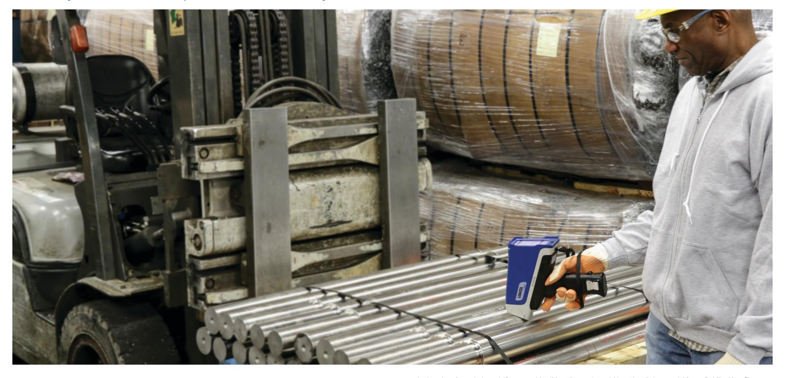
As the price of recycled metals fluctuates, identifying alloy grades quickly and easily is essential for profitability. Vanta<sup>™</sup> handheld XRF analyzers for scrap sorting provide reliable identification in seconds for most alloys and pure metals.
