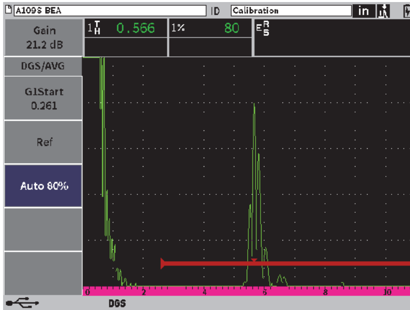
Figure 11-20 Reference reflector before capture
