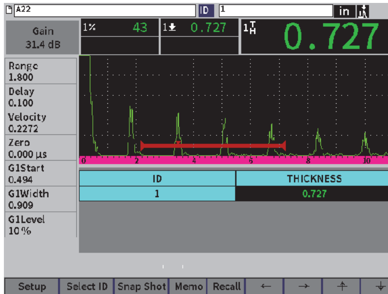
Figure 9-27 Grid controls in a saved file
