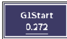
Figure 4-3 Enhanced border indicates selected adjustable value
