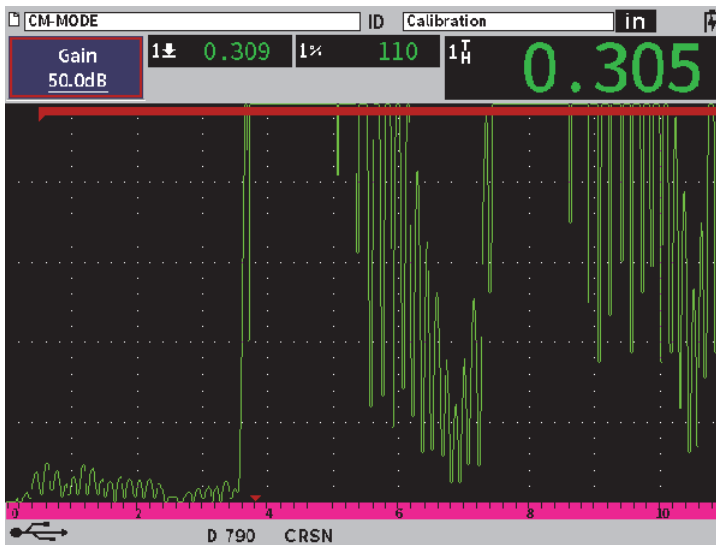
Figure 11-39 Adjust gain value in precision mode
