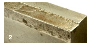
Severe fretting corrosion and material removal of a WT gearbox key, which caused shaft cracking.
