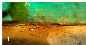
Hematite wear debris emerging from the interface between the main bearing housing and a bedplate.
