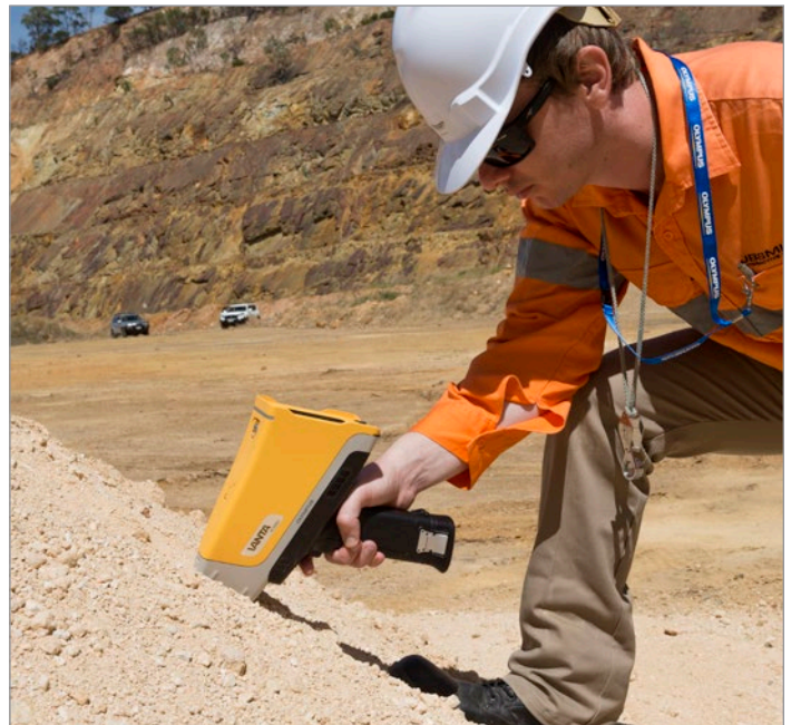
A Vanta pXRF analyzer being used to sample stockpiles
