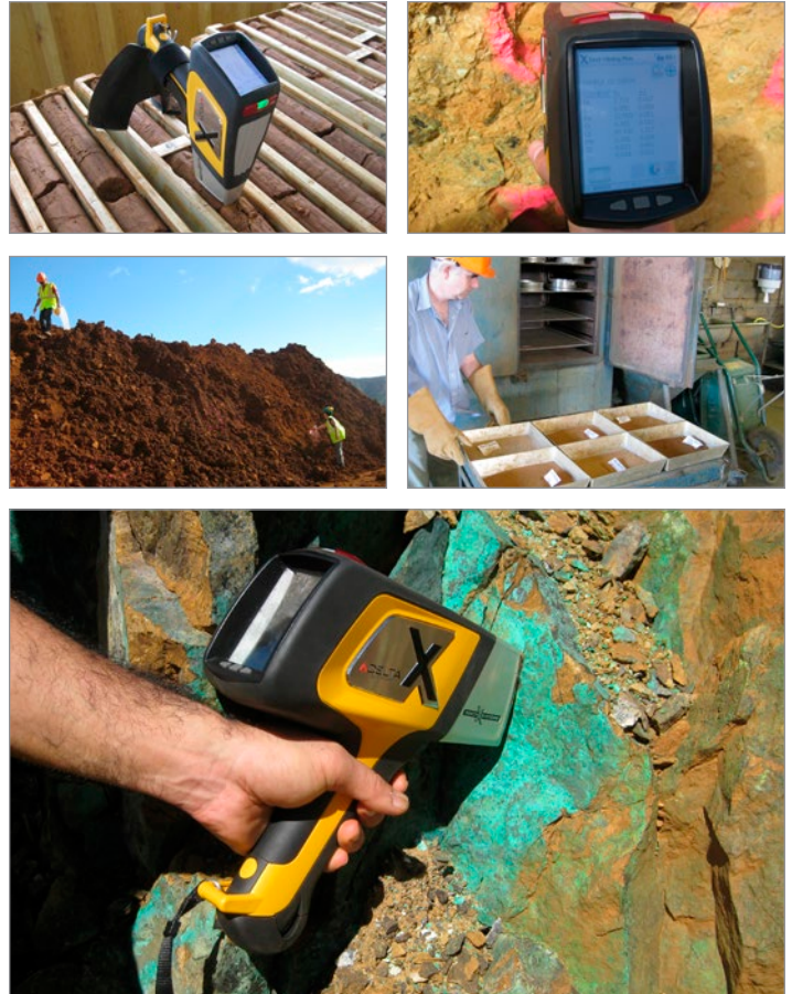
Field photos showing the various use cases for pXRF on a nickel laterite project: On diamond drill core, face sampling, stockpile sampling and concentrates in the laboratory
