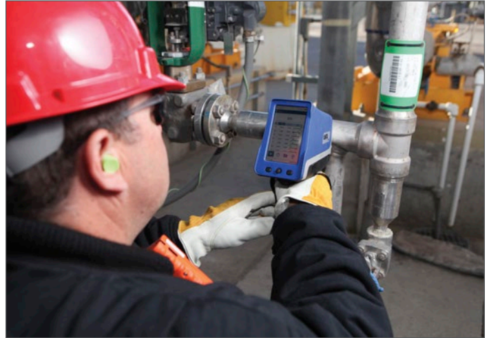
Figure 1—XRF technology enables fast, convenient PMI measurements of pipes and other components.
