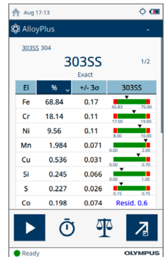
Figure 3—The Vanta analyzer's precise, reliable readouts make it easy to determine the composition of an alloy.
