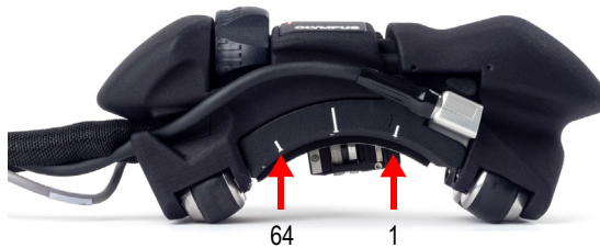
Figure 4-5 Probe element marks on the wedge
