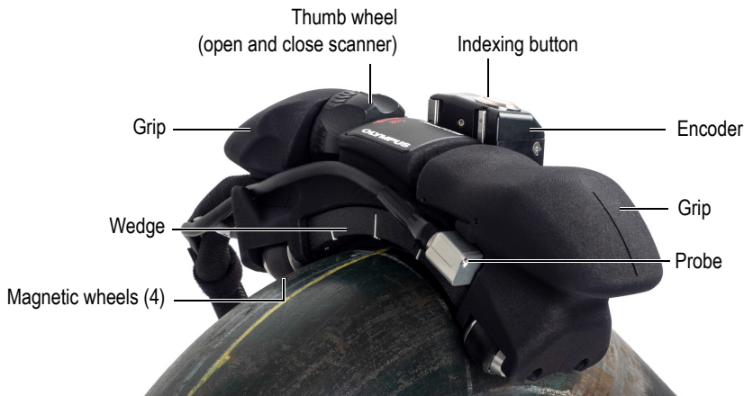
Figure 1-2 Scanner components
