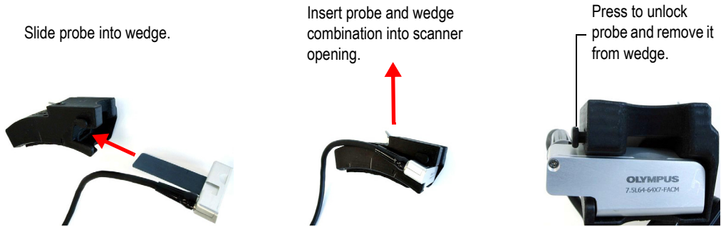
Figure 2-3 Installing the probe and wedge
