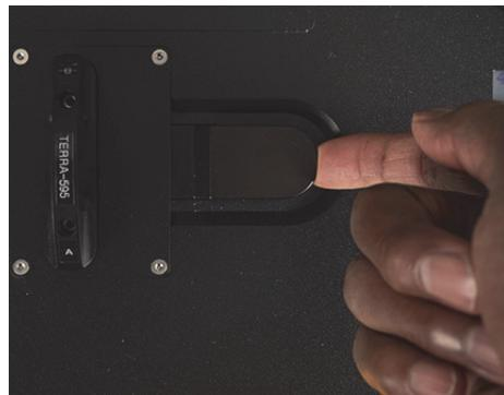
2. Pull up the carrier handle to remove the sample carrier.
