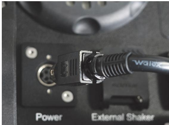
2. Plug one end of the AC power cord firmly into the power supply.
