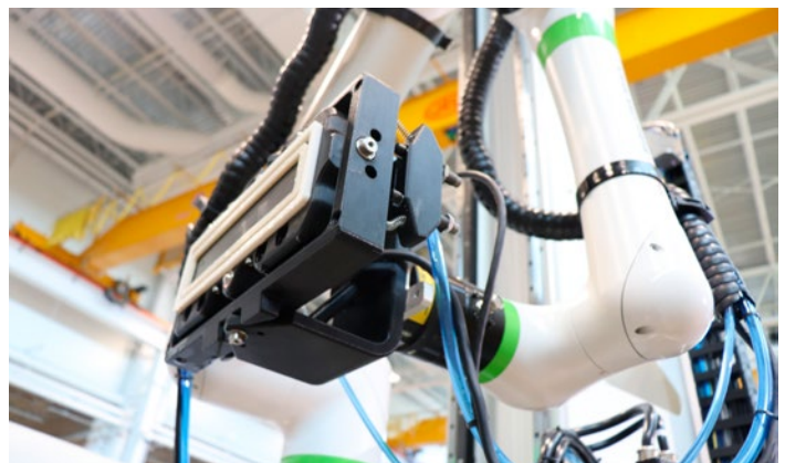
Phased array probe and water wedge mounted on the cobot arm of an AGV, also equipped with a FOCUS PX data acquisition unit (not showing)
