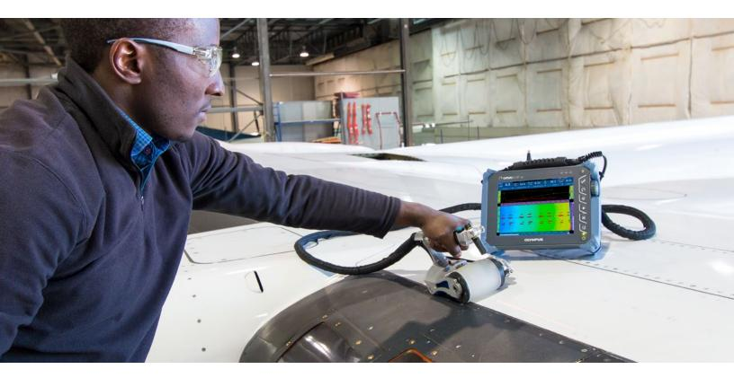
The RollerFORM™ phased array wheel probe from Olympus is designed to address the inspection of composites and other smooth-surfaced materials. An affordable and easy-to-implement replacement for full 2D encoding systems, the RollerFORM scanner is a viable alternative to immersion techniques.
