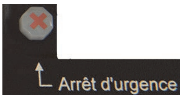
Figure 1-4 Stop/Emergency Shutoff button
