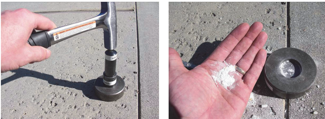
Figure 3-4 Crushing a sample
