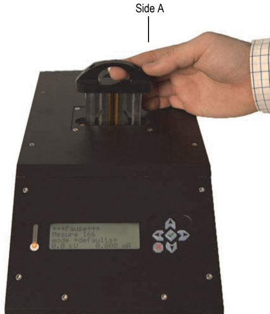
Figure 3-15 Inserting the sample carrier
