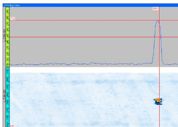
Figure 6: Inspection results for longitudinal OD defects
