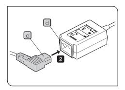
2 Insert the power cord connector © in the connector d of the AC adapter.
