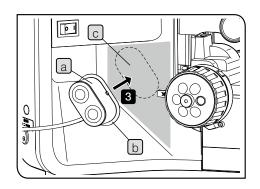
This picture shows the procedure to attach the hand switch for motorized nosepiece (BX3M-HSRE). The same procedure applies when attaching the hand switch for exposure (U-HSEXP).
