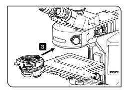
3 Insert the nosepiece from the front side along the nosepiece mounting dovetail of the reflected light illuminator, and push it until it touches the end. When attaching the coded nosepiece, put the cable a for the nosepiece through the cable hole b on the top of the microscope frame, and put it out to the back of the microscope frame.
