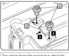
This picture shows the procedure to attach the cable for motorized nosepiece to the microscope frame. The same procedure applies when attaching it to the height adapter.
