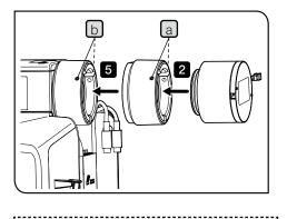
This picture shows the procedure to attach the reflected LED lamp housing (BX3M-LEDR). The same procedure applies when attaching the mercury lamp housing.
