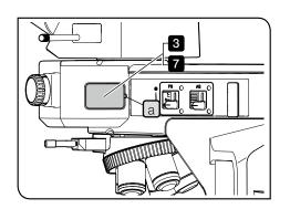
3 Insert a stick with a fine point, such as a precision screwdriver, etc. in the notch a and catch the cover to remove it.
