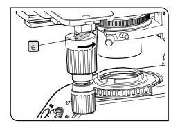
) If it is too tight to raise the Y-axis knob b in 1. lock the stage movement with the Y-axis lock lever e once, and turn the Y-axis knob b to raise the Y-axis knob.
