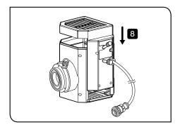
8 Align the external surfaces of the lamp housing with those on the socket part, push the lamp housing straight downward and place the socket part to the original position.
