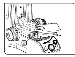
**3** Turn the filter cassette so that the filter cassette is parallel to the base unit.
