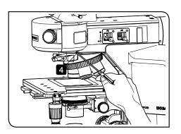
4 Hold the Allen screwdriver between the pointing finger and the thumb, and tighten the nosepiece clamping screw to secure the nosepiece.
