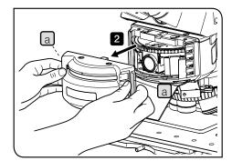
2 Hold the both sides of the cover a on the front of the illuminator lightly and pull it to the front side.
