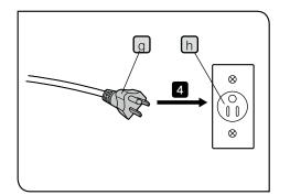
4 Connect the power cord plug g to the power outlet h. (Perform this operation for both power cords of the AC adapter connected to the control box and the AC adapter connected to the microscope frame.)
