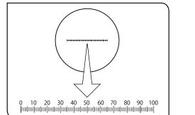
4 Turn the diopter adjustment ring b of the eyepiece not equipped with the eyepiece micrometer to bring the sample into focus.
