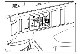
TIP Before performing centering, turn ON the main switch of the power supply for mercury lamp housing and wait until the illumination light does not flicker and the brightness becomes stable.
