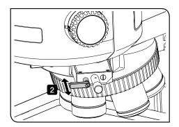
2 When using the DIC slider U-DICR, slide the selection lever depending on the objective to use.
