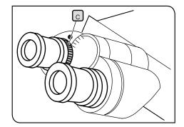
When the observation tube is equipped with the interpupillary distance adjustment ring **C**
