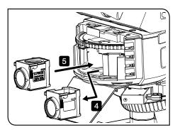
4 Hold the side of the fluorescence mirror unit to be replaced, and pull it to the front side to remove it.
