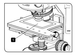
1 Place the sample on the stage plate or the holder plate before observation.
