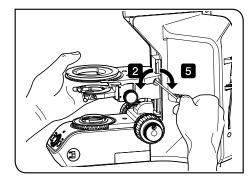
While holding the stage holder, loosen the clamping screw of the 2 stage holder.
