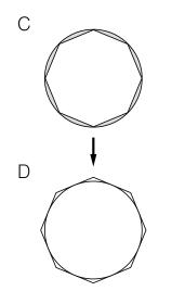
5 Move the field diaphragm knob (field diaphragm lever) to open the field diaphragm image until the field diaphragm image inscribes to the field of view. (Picture C) If the field diaphragm image is decentered, try centering again.
