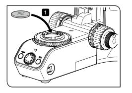
Inserting the filter in the filter mount
