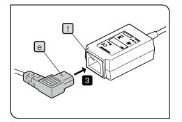
3 Insert the power cord connector e in the connector f of the AC adapter. (Perform this operation for both the AC adapter connected to the control box and the AC adapter connected to the microscope frame.)
