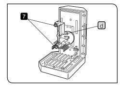
6 Hold the new mercury burner wrapped with gauze, etc. and attach the + (positive) pole of the mercury burner d to the fixed mount on the upper side, then attach the - (negative) pole to the mount on the lower side.
