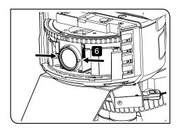
6 Hold the both sides of the inserted fluorescence mirror unit between the thumb and the pointing finger, and swing it from side to side lightly to confirm that the fluorescence mirror unit is secured firmly. Without this operation, the fluorescence mirror unit may be attached being tilted.
