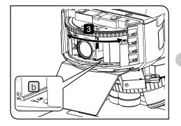
3 Turn the turret until the position number b of the fluorescence mirror unit to be replaced comes to the front side, and stop it when the clicking sound is heard.
