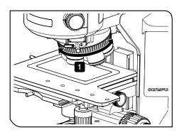
NOTE When selecting the objective, be careful not to collide with the sample.
