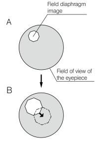
3 Move the field diaphragm knob (field diaphragm lever) of the reflected light illuminator to narrow down the diameter of the field diaphragm image to the minimum approximately. (Picture A)
