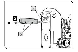
2 Align the screw holes (2 positions) on the bottom of the microscope frame with the mounting holes (b) (2 positions) of the overturing prevention plate, and tighten the provided screws to secure the overturing prevention plate.
