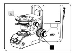
Turn the coarse focusing knob to lower the stage holder c sufficiently.
