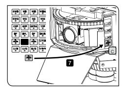
7 Insert the indicator sheet corresponding to the fluorescence mirror unit which was inserted in **5** in the inscription pocket **C**. The indicator sheet is provided with BX3M-URAS-S.
