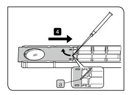
4 Insert the precision screwdriver in the notch a, and raise and slide the cover with the precision screwdriver to return the cover to the original position. At this time, slide the cover under the tabs (6 positions) c until the "clap" sound is heard.
