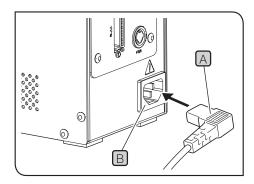
1 Insert the power cord connector A in the connector B of CMP-CB.
