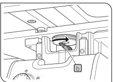
Pull out the eyepiece. While looking into the eyepiece sleeve, rotate the aperture diaphragm lever toward right side. (At this time, narrowing down the aperture diaphragm to 70% to 80% allows you to obtain the image with good contrast.)
