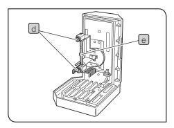
6 Hold the new mercury burner wrapped with gauze, etc. and attach the + (positive) pole of the mercury burner e to the fixed mount on the upper side, then attach the - (negative) pole to the mount on the lower side.
