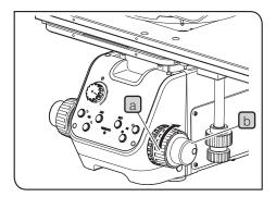
1 Rotate the coarse focusing knob a and the fine focusing knob in the arrow direction to move the stage upward. (The sample approaches the objective.)
