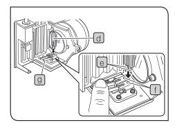
While pressing down the bulb fixing lever d, hold the halogen bulb wrapped with gauze, etc. and insert the terminal f until it touches the pin position g.
