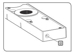
Layout of the cable for MIX slider for reflected light observation
