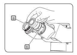
1 Pull out the eyepiece a from the eyepiece sleeve b.
