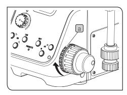
The tension of the coarse focusing knob is pre-adjusted for easy use, but if you wish, you can change the tension. Rotating the coarse focusing tension adjustment ring a in the arrow direction increases the tension and in the opposite direction decreases the tension.
