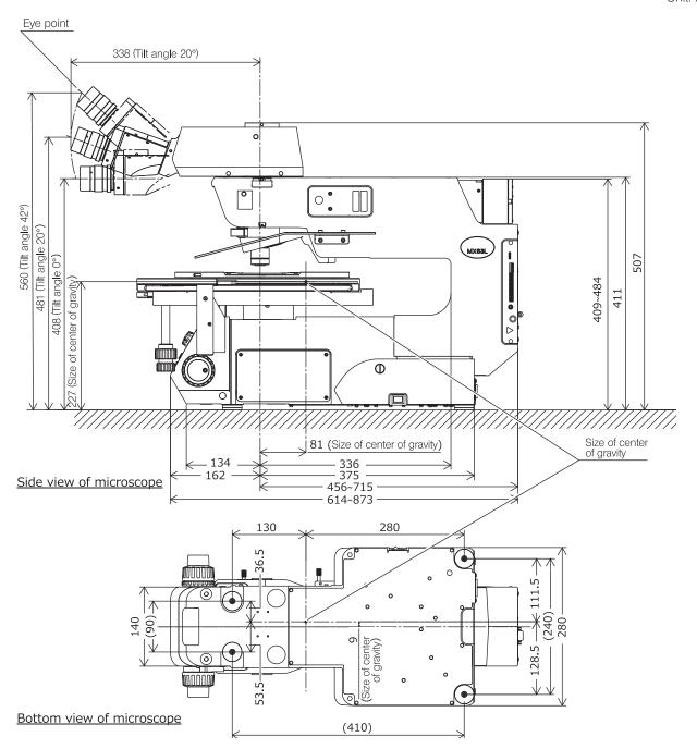
TIP The center of gravity is an approximate position in the standard combination for transmitted light observation. Note that the position varies depending on the sample weight, stage position and other units to be combined.
