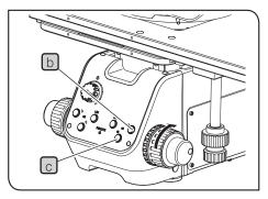
The aperture diaphragm is used to adjust the numerical aperture of the illumination system. Matching the numerical aperture of the illumination system with that of the objective to be used offers an image with optimum contrast and also increases the focal depth of image. However, this adjustment may decrease the resolution and brightness. In general, adjusting the numerical aperture to 70% to 80% of that of the objective allows you to obtain a well-balanced image.
