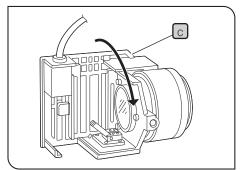
3 Tilt the lamp socket c in the arrow direction by 90°.
