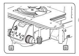
Rotate the light intensity knob a counterclockwise fully and set the main switch to (ON).
