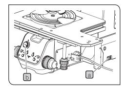
1 Set the main switch a of the microscope frame to (ON), and rotate the light intensity knob b counterclockwise completely.
