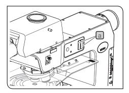
1 Insert the filter slider suitable for the intended observation into the filter insertion slot (2 positions) a to engage in the light path. The first level (position where the clicking sound is heard first) is an empty hole. The filter is engaged in the light path at the second level (position where the clicking sound is heard next).
