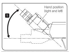
The picture shows the hand position when adjusting the tilt of MX-SWETTR. (Same for other observation tubes.)
