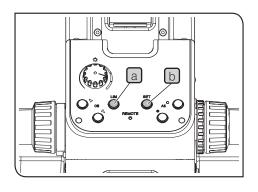
Restoring the stored brightness (LIM function) to the factory default setting
