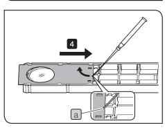
Insert the precision screwdriver in the notch a, and raise and slide the cover with the precision screwdriver to return the cover to the original position. At this time, slide the cover under the tabs (6 positions) until the "clap" sound is heard.
