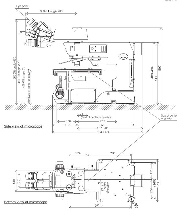
TIP The center of gravity is an approximate position in the standard combination for transmitted light observation. Note that the position varies depending on the sample weight, stage position and other units to be combined.
