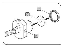
Attaching the filter at the tip of light guide
