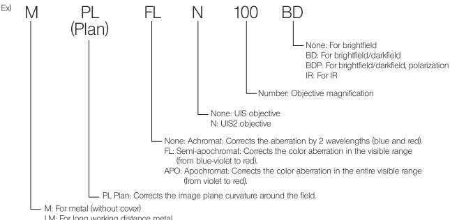
LM: For long working distance metal SLM: For super long working distance metal
