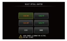
Select the optical adapter to use, and press the [MEAS/ENTER] joystick.
