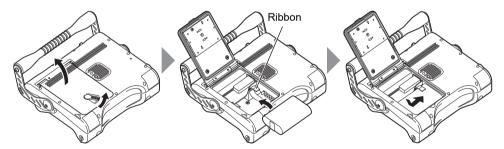
Slide the lock release lever to the side to open the battery cover.
