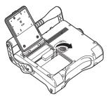
If you find it difficult to remove the battery, hook your finger directly onto the battery to remove it.
