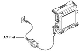
After connecting the AC power cord to the AC inlet of the AC adapter, plug the plug end of the AC power cord securely into a 3P power outlet.
