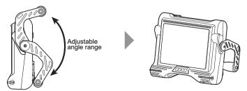
When installing the main unit on a flat surface for observation, use the handle as a stand. Adjust the handle to an angle that allows the LCD monitor to be easily viewed. The angle of the handle can be adjusted smoothly to any position within the range shown in the figure above.
