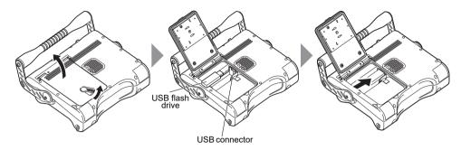
Slide the lock release lever to the side to open the battery cover.
