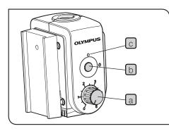
NOTE Before turning ON the main switch of the compact light guide illuminator SZ2-CLS, set the light intensity control knob a to "0".
