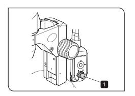
1 Rotate the light intensity control knob to adjust the brightness. Rotating the light intensity control knob in the clockwise direction makes the illumination brighter and rotating it in the counterclockwise direction makes the illumination darker. Light guides
