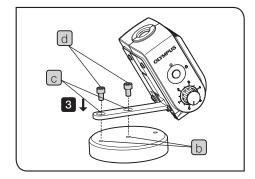
3 Match the screw holes (2 positions) of the CLS stand SZ2-CLSST with the mounting holes (c) of the adapter which was combined in (2), and tighten the provided screw (d) using the Allen wrench provided with the illuminator SZ2-CLS to secure the illuminator.
