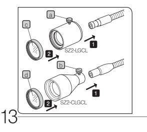
1 Loosen the clamping screw a or b of the collector lens. Insert the collector lens into the output end of the light guide completely and when it touches the end, tighten the clamping screw a or b.
