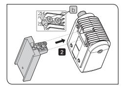
2 Combine the adapter with the illuminator SZ2-CLS and tighten the bottom screws b (2 positions). Tighten screws so that the washer (resin ring) is placed between the illuminator and the adapter.
