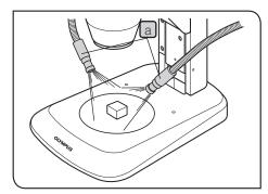
Hold the output end **a** of the light guide with a hand and irradiate the light on the specimen from the position that does not interrupt the observation. Do not twist the light guide as much as possible.
