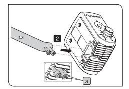
2 Combine the CLS stand adapter SZ2-CLSSTAD with the illuminator SZ2-CLS and tighten the bottom screws a (2 positions).
