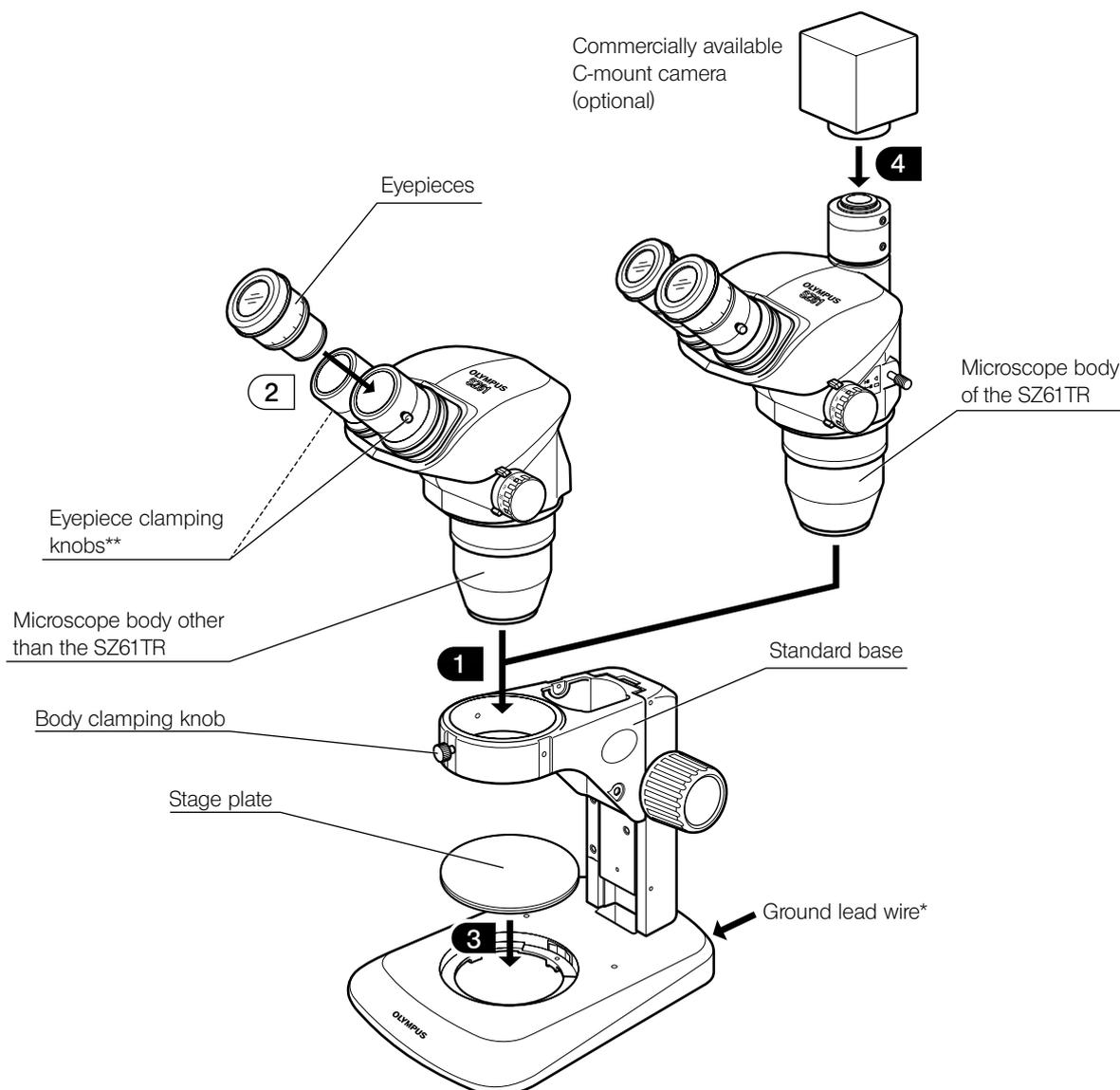
\* To reserve the ESD protection performance, be sure to ground the equipment using a grounding lead wire having a 4 mm banana plug.
