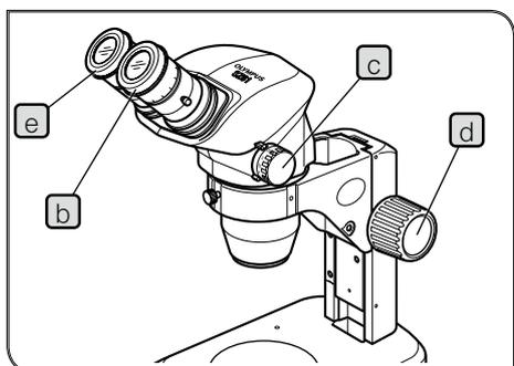
Eyepieces with eyepiece micrometer disk
