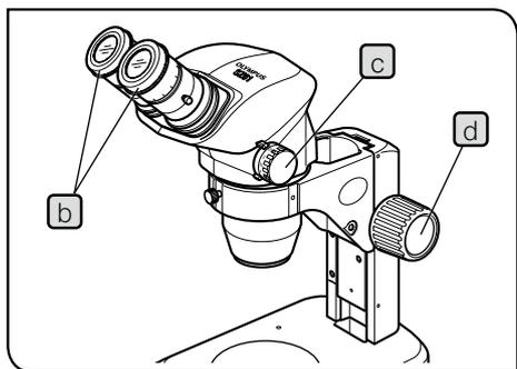
Eyepieces without eyepiece micrometer disk
