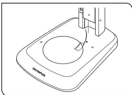
**TIP** To fix a container such as a petri dish, insert the provided tube into the specimen holder to fix the container by pinching.
