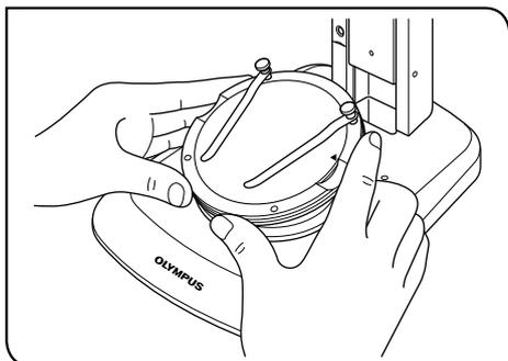
Place a specimen on the stage plate, hold the cup stage by the edge, and tilt the cup stage slowly.
