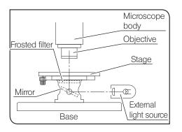
1 Illuminate the specimen with an external light source (LSD illuminator, light guide illuminator, etc.).
