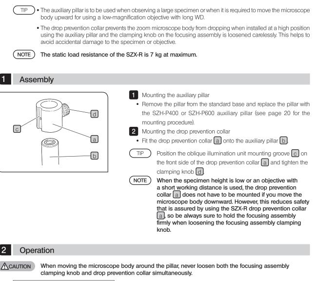
To Move the Microscope Body Upward
