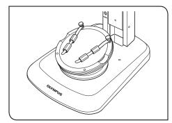
To fix a container such as a petri dish, insert the provided tube into the specimen holder to fix the container by pinching.
