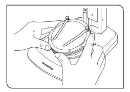
1 Place a specimen on the stage plate, hold the cup stage by the edge, and tilt the cup stage slowly.
