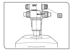
2 Return the microscope body to the illumination light path by loosening the focusing module clamping knob **b**, rotating the microscope body gently in the direction of the arrow, aligning visually the objective with the illumination light path and tightening the clamping knob **b** again. Now the setting of the photo light path is complete.
