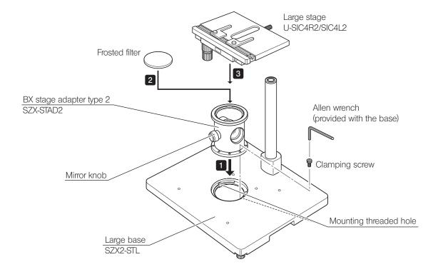
NOTE For simplified transmitted light observation, place the mirror knob on the front and use a frosted filter.
