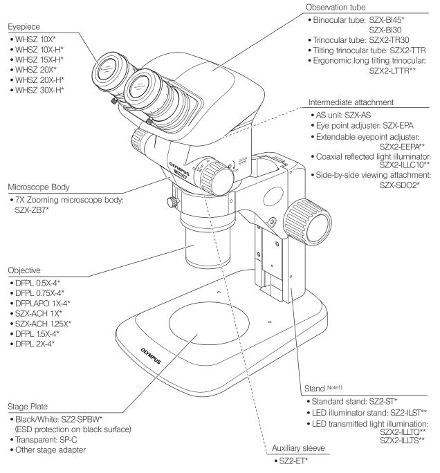
Note1) The microscope can also be mounted on the SZ2-STU1/STU2/STU3 large stand as well as on the SZX2-ST SZX standard stand by using the SZ2-STB1/SZ2-STS focusing arm.
