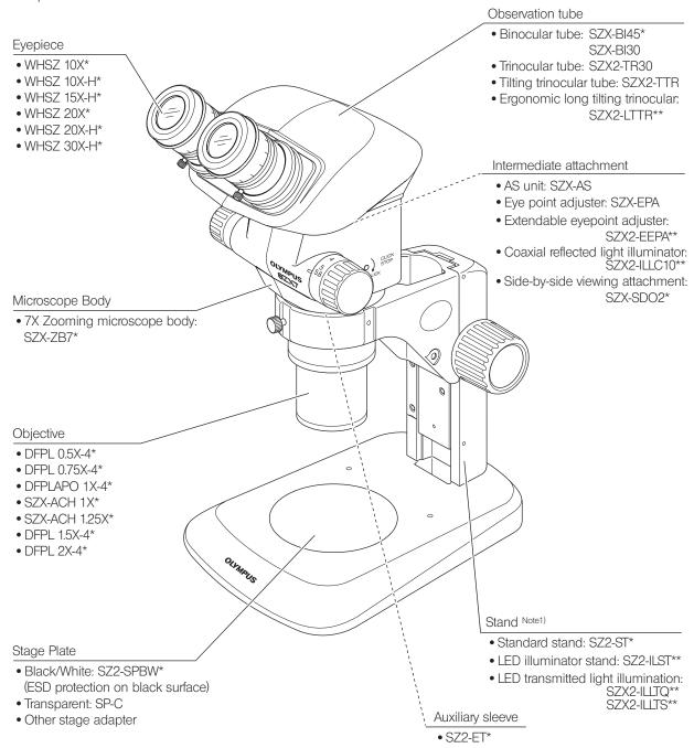
Note1) The microscope can also be mounted on the SZ2-STU1/STU2/STU3 large stand as well as on the SZX2-ST SZX standard stand by using the SZ2-STB1/SZ2-STS focusing arm.
