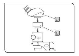
1 Remove the observation tube a using the Allen screwdriver provided with the SZX microscope body.
