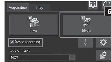
**6** Record the movie. Check the [Movie recording] checkbox. Press the [Movie] button to start recording the movie. To stop recording, press the [Stop Movie] button in the dialog box displayed on the live image.
