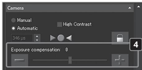
**4** Adjust the brightness. Press the or button in [Exposure compensation]. If the specimen is too dark, perform "+ compensation". If the specimen is too bright, perform "- compensation".
