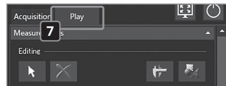
**7** Check the acquisition results. Select the [Play] tab and check the acquisition results. (See the reverse side for details.)
