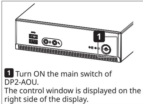
**1** Turn ON the main switch of DP2-AOU. The control window is displayed on the right side of the display.
