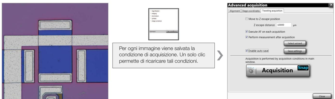
The image shows the 'Advanced acquisition' software interface with the 'Traveling acquisition' tab selected. It displays various settings for acquisition, including 'Execute AF on each acquisition' and 'Perform measurement after acquisition' checked. A 'Snap' button is visible at the bottom.
