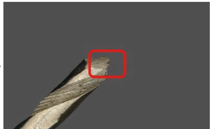
Easy observation (24X) of damaged area with DSX1000 thanks to the flat lighting
