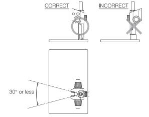
· When attaching the focusing assembly on the top of the pillar of the SZX2-STL2 base, be sure to insert the SZX-R drop prevention ring (optionally available) immediately below the focusing assembly without leaving any clearance.
