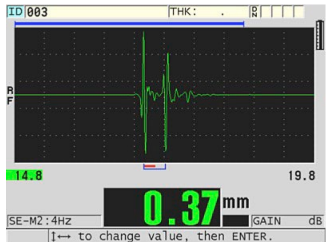
Plastic tubing: 2 mm (0.080 in.) diameter, 0.37 mm (0.014 in.) wall thickness
