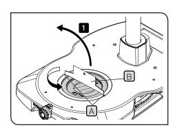
Insert the screwdriver B for stage glass frame provided with the base into the notch A of the stage glass frame, and rotate it in counterclockwise direction to remove the stage glass.
