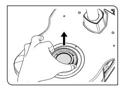
TIP When removing the illumination cartridge, pull the illumination cartridge up and remove it.
