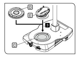
Attaching SZH-SG (Gliding stage) or SZH-SC (Cup stage)
