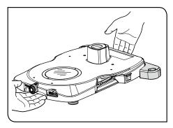
4 Flip the base back to its front and place it down carefully.
