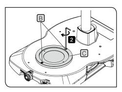
2 Securing the screws (2 pcs.) B to the screw holes (2 positions) of the base using the Allen wrench, attach SZX2-STADM (STAD mount for ILLT) C to the base.
