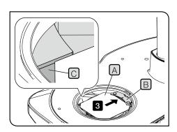
1 Cut the four corners of the photo sheet filter by approx. 10 mm using the scissors.
