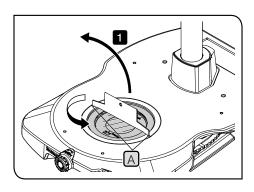
1 Insert the screwdriver for stage glass frame into the notch A of the stage glass frame, and rotate it in counterclockwise direction to remove the stage glass.
