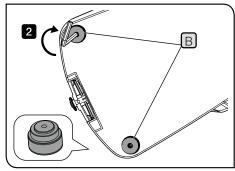
2 Securing the screws attached to the provided rubber legs (2 pcs) B to the screw holes (2 positions) used for attaching the rubber legs (2 pcs.) A using the Allen wrench, attach the provided rubber legs (2 pcs.) B
