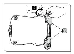
3 Securing the screws (4 pcs.) to the screw holes (4 positions) at the back of the base using the Allen wrench, attach SZX2-ILLTSA (High stability adapter for ILLT) C
