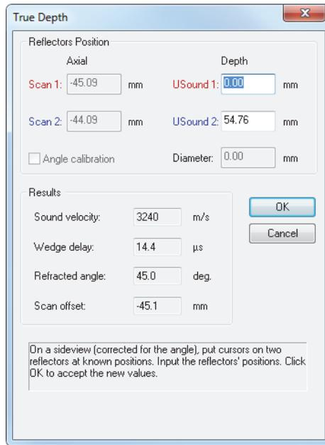
Figure 2-7 The calibration dialog box in True Depth mode
