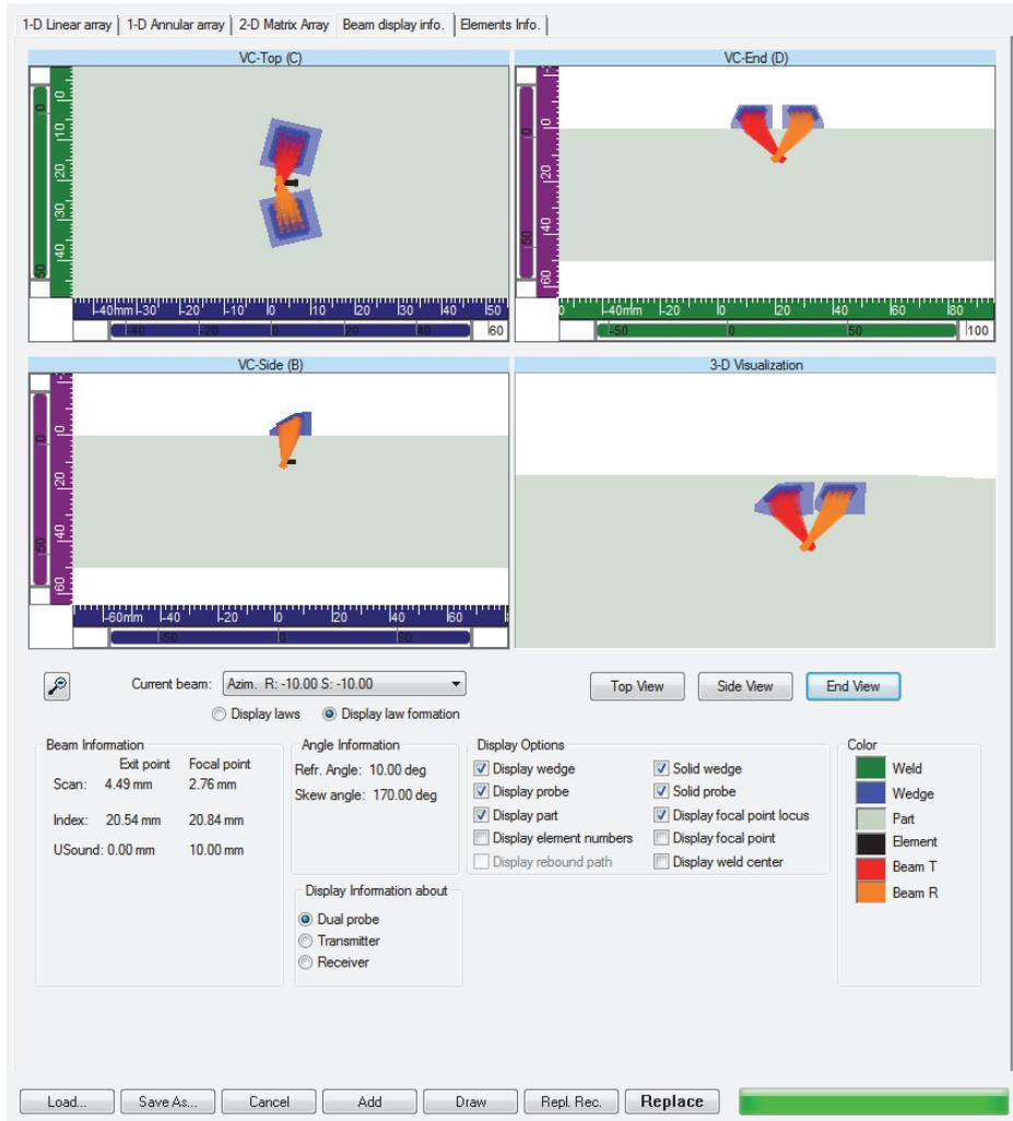
Figure 10-2 Graphic representation of the sectorial beams for a 2-D matrix probe
