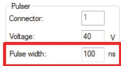
The image shows a screenshot of the 'Pulser' section within the 'UT Settings' dialog box. It contains three input fields: 'Connector' with the value '1', 'Voltage' with the value '40' and a 'V' unit indicator, and 'Pulse width' with the value '100' and a 'ns' unit indicator. A red rectangular box highlights the 'Pulse width' field and its unit.
