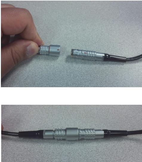
Figure 2-9 Joining the sections of the encoder cable
