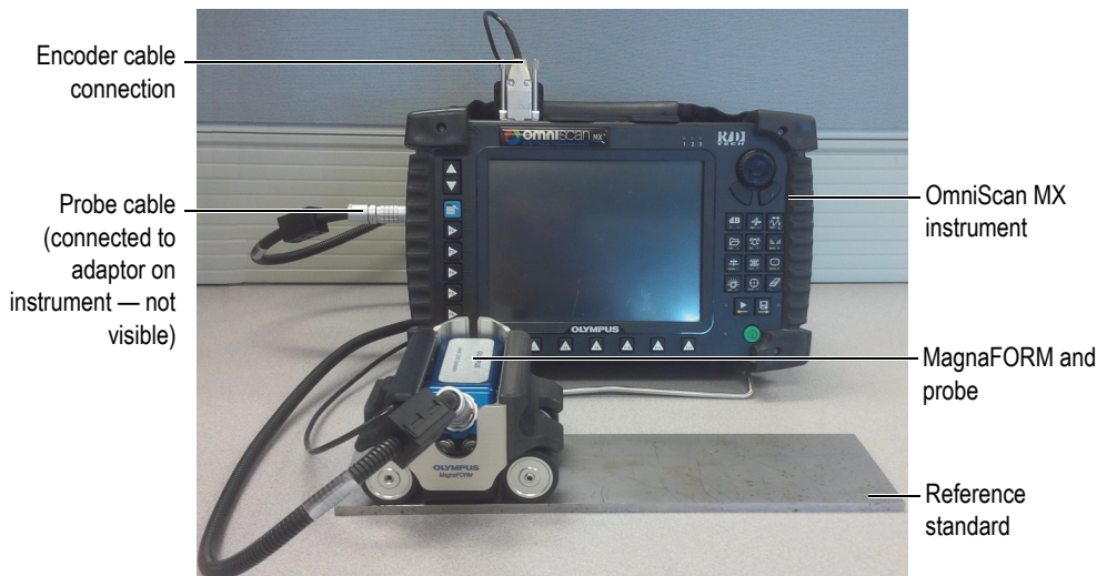
Figure 1-1 An example of an inspection setup
