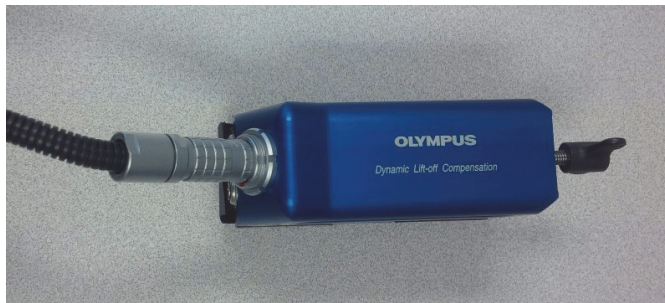
Figure 2-7 Connecting the cable to the probe
