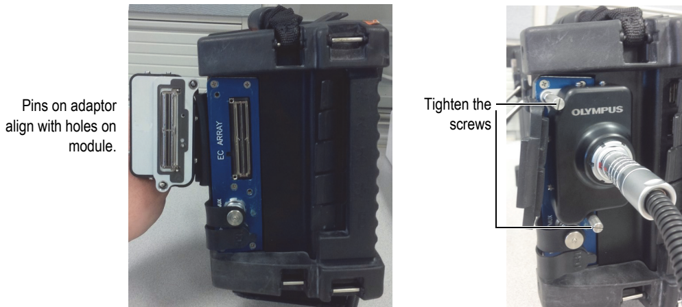
Figure 2-11 Connecting the adaptor to the OmniScan MX
