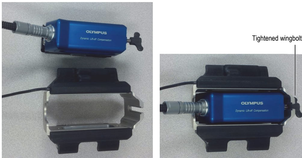
Figure 2-8 Installing the probe onto the MagnaFORM
