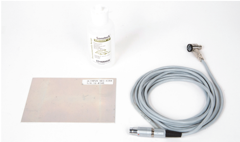
Figure 6-37 Materials — metal-to-metal bonds using resonance technique
