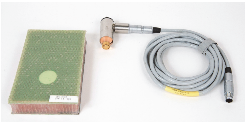
Figure 6-29 Materials — repaired areas (potting) using MIA technique
