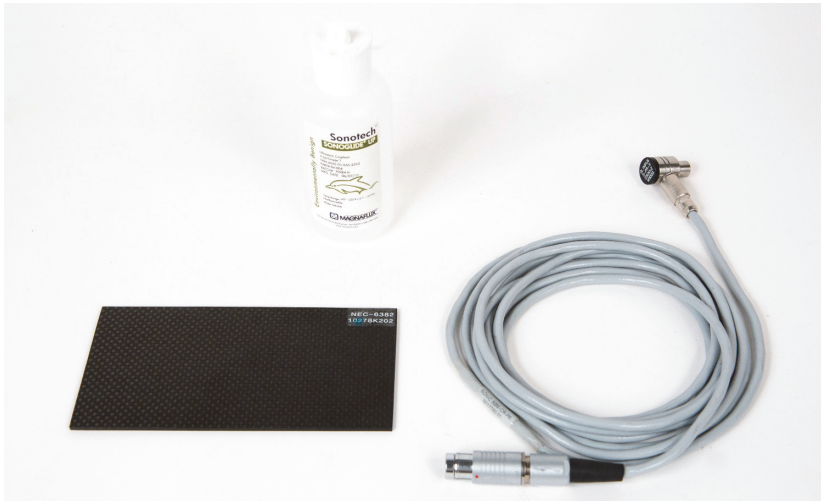
Figure 6-45 Materials — delamination in composites using resonance technique
