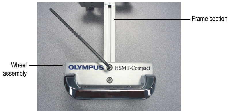
Figure 2-4 Loosening the wheel assembly
