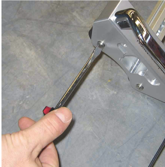
Figure 4-1 Removing the wheel screw
