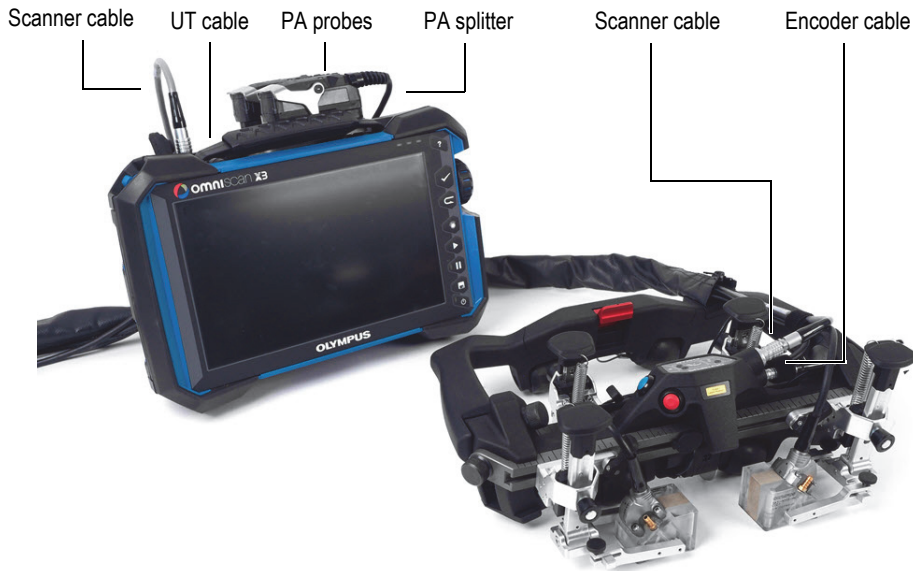
Figure 2-28 Scanner and OmniScan connected
