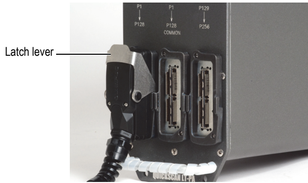
Figure A-3 Phased array connector with latch
