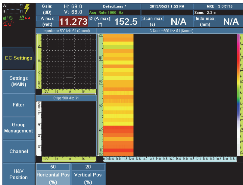
Figure 13-27 Setting the horizontal and vertical positions of the offset null in the impedance plane view
