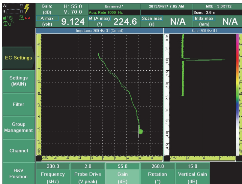
Figure 13-2 Adjusting the gain of the deepest crack signal
