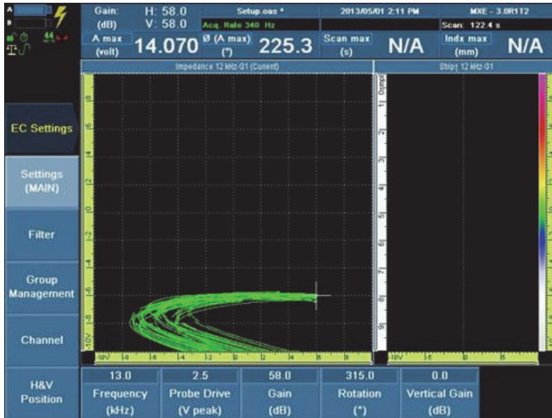
Figure 13-11 Adjusting the Rotation parameter to orient the signal horizontally
