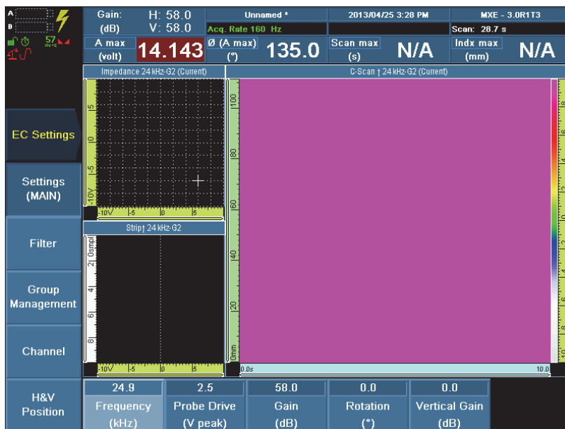
Figure 9-22 Configuring the Frequency and Gain parameters for mixing frequency 2
