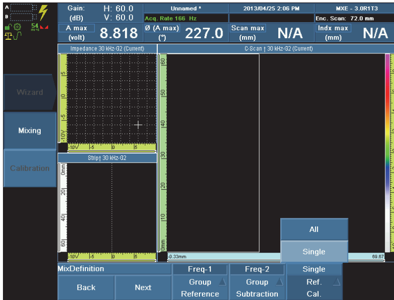
Figure 9-10 Setting the Ref. Cal. parameter to Single
