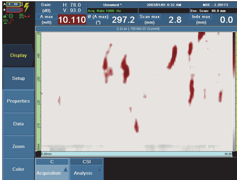
Figure 12-5 The C-scan view with a 1:1 ratio in C-scan view mode
