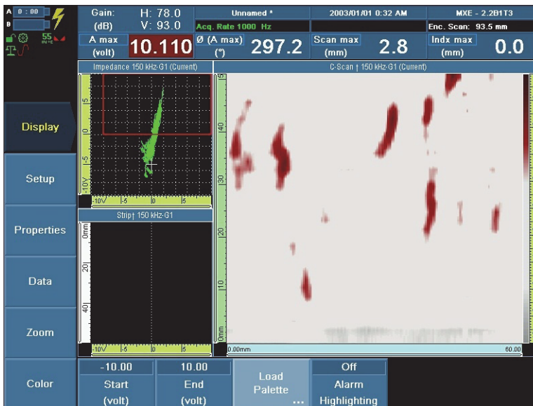
Figure 12-4 The C-scan view displayed with a 1:1 ratio in CSI view mode
