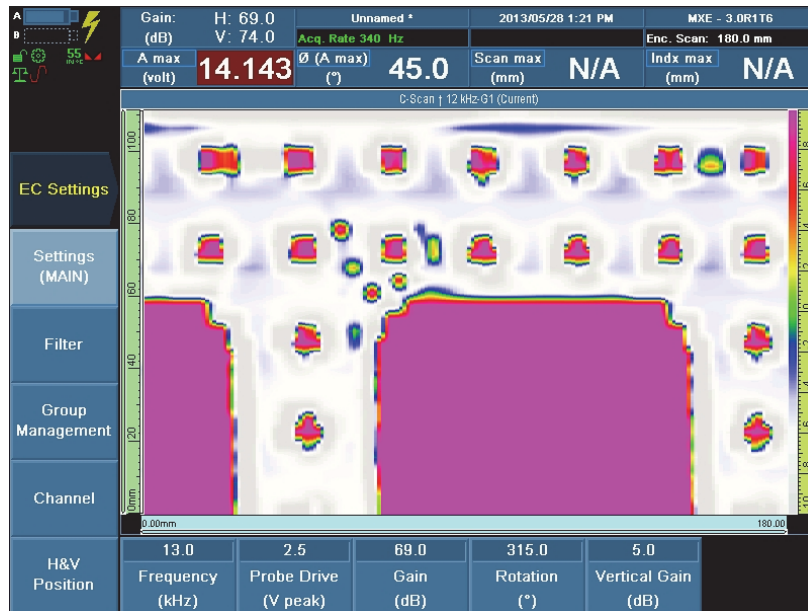
Figure 13-16 Typical example of corrosion inspection on a RSTD-10123 validation standard
