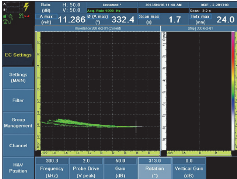
Figure 13-5 Setting the Rotation parameter to orient the signal horizontally
