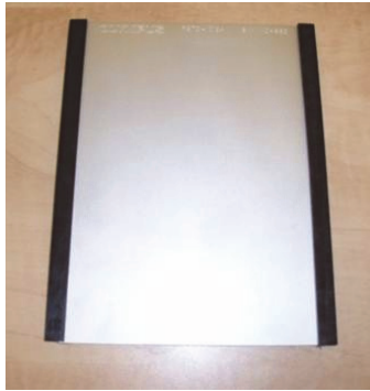
Figure 13-10 The calibration assembly for ECA corrosion inspection
