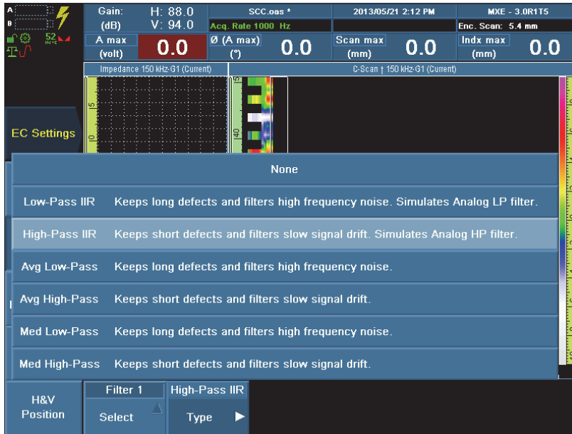
Figure 13-39 Configuring the High-Pass IIR filter
