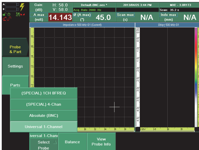
Figure 9-34 Selecting the probe for mixing in ECT mode
