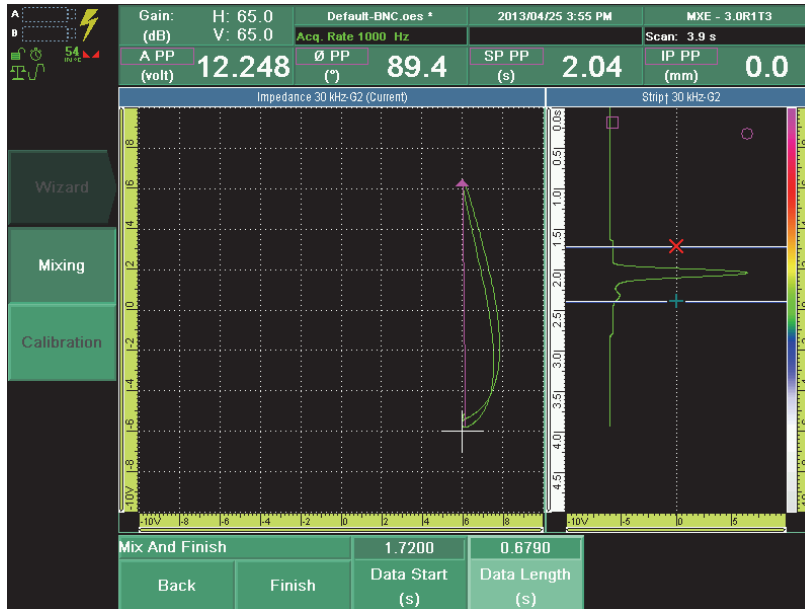
Figure 9-42 Positioning the measurement cursors in the Mix and Finish step
