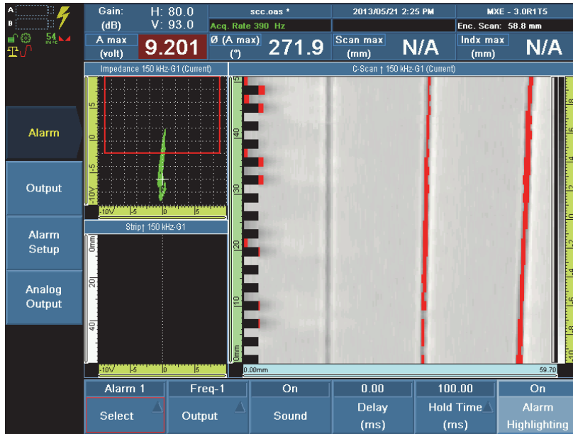
Figure 13-42 Alarm activated for the accept/reject criteria
