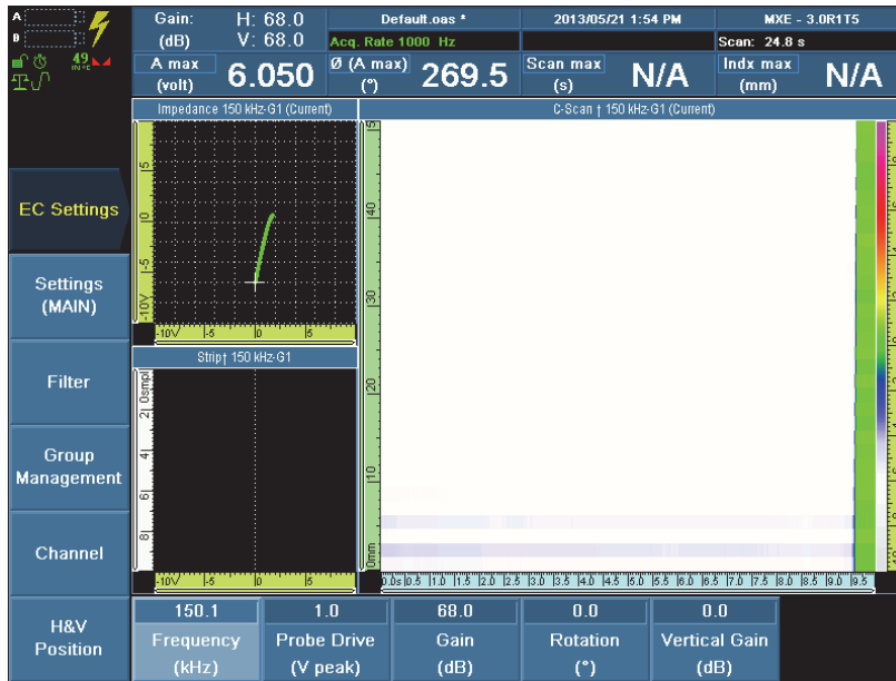
Figure 13-28 Setting the frequency for stress corrosion cracking detection on carbon steel piping
