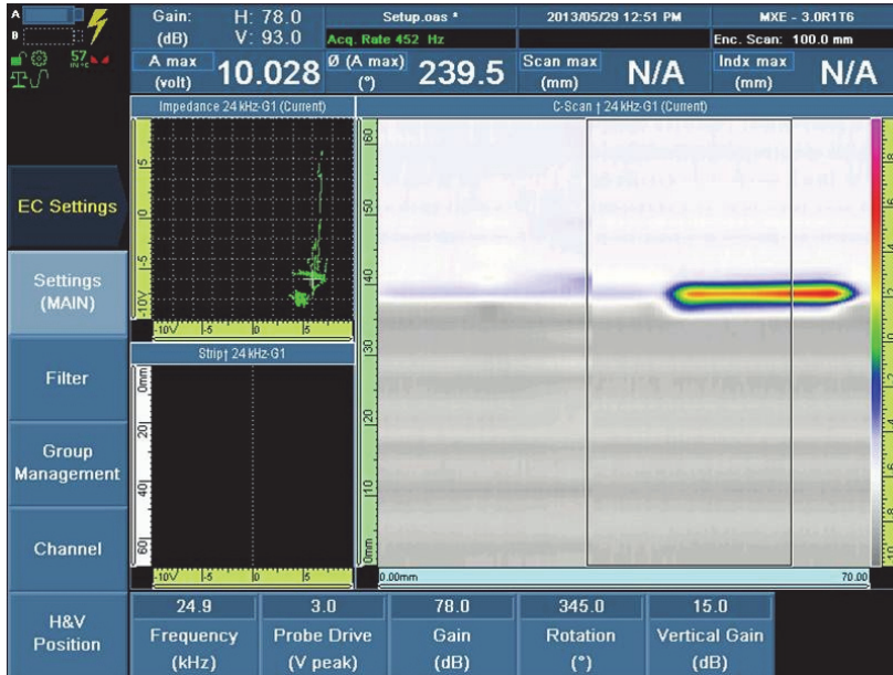
Figure 13-24 Crack and doubler signals displayed on the C-scan
