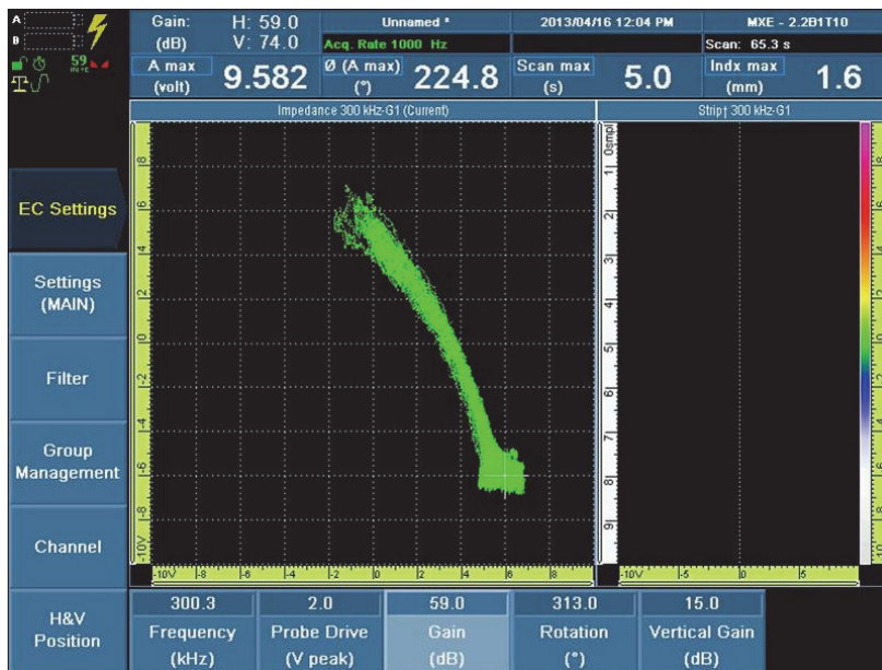
Figure 13-6 Setting the Gain parameter to expand the signal vertically
