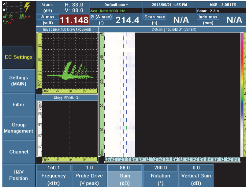
Figure 13-30 Adjusting the gain to expand the signal of the defects
