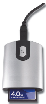
Figure 4-11 Example of a storage card and reader
