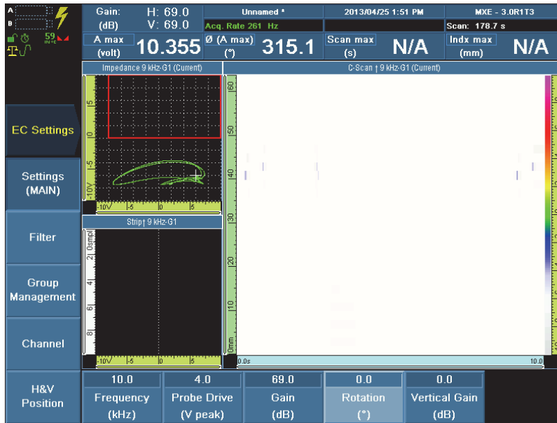
Figure 9-3 The defective fastener’s signal using mixing frequency 1
