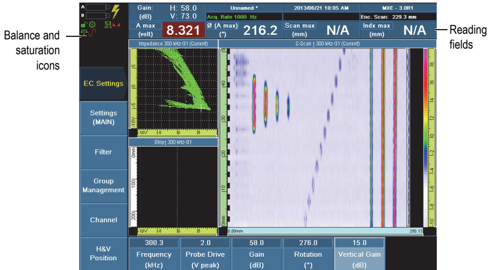
Figure 2-3 The reading fields and icons at the top of the OmniScan MX display
