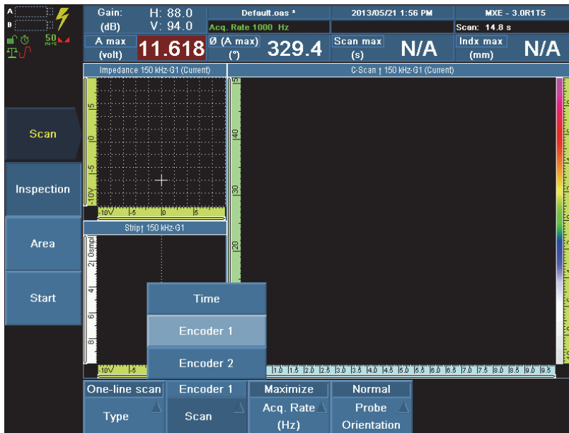
Figure 13-32 Activating the probe encoder
