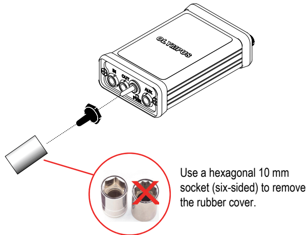
Figure 3-1 Replacing the switch’s rubber cover
