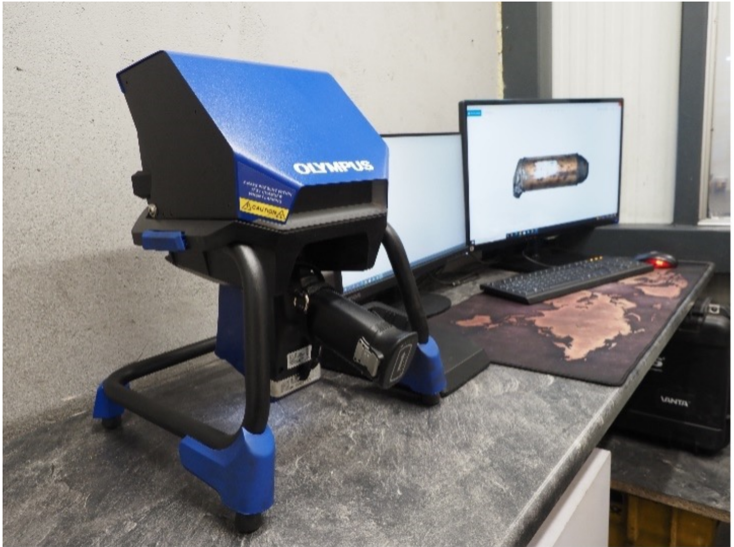
Figure 5: Analysis of the catalyst sample using a Vanta VLW analyzer and Vanta Work Station
