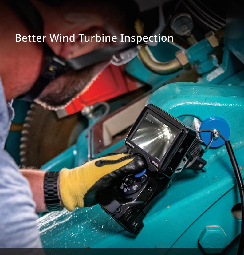
If you're inspecting in the cramped quarters of a wind tower nacelle, the wind version of the IPLEX G Lite videoscope's combination of portability and powerful imaging features packed into a small body can make your job easier. This version of the IPLEX G Lite has features designed specifically for wind tower inspection, such as:
