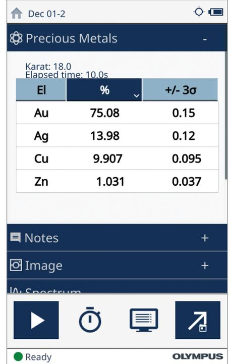
The screenshot shows the Vanta GX software interface. At the top, it displays 'Dec 01-2' and 'Precious Metals'. Below this, it shows 'Karat: 18.0' and 'Elapsed time: 10.0s'. A table lists the following results:
